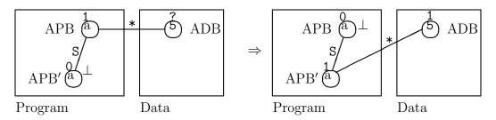
Note: the APB-ADB bond \* has moved: Before execution, it connected APB with ADB. After execution, it connects APB' with ADB, where APB' is the next instruction: the successor (via bond S) of the previous APB. Also note that the activation bit has changed: before, it was 1 at APB (indicating that the APB was about to be executed) and 0 at ADB'. Afterwards, those two
